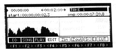
When you enter this page, you see a graphic representation of the takes waveform and you may move the start and end points around freely. The start and end points are shown both as time values in the START and END fields respectively and are also shown as flashing vertical lines in the waveform display. You may zoom in or out on a waveform for greater editing accuracy. The fields are as follows:
