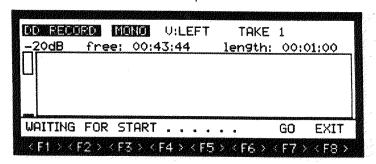
Here, the S1100 is either waiting for a MIDI NOTE or a SONG START command or for the footswitch to be triggered or the input level to exceed the threshold level. This all depends on the type of START you have selected in DREC. You may manually initiate a recording by pressing GO (F7). You may get out of this display by pressing EXIT (F8).
