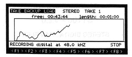
This is virtually identical to the normal record page when a recording is being made and the takes waveform envelope will be displayed as it is being restored. The DAT restore function is, actually, just another way of recording and this 'confidence monitoring' keeps you informed of progress during the DAT restore process. At any time, you may press STOP (F8) to abort the restore.
