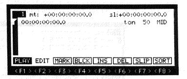
The note number and MIDI velocity parameters are replaced with level and pan parameters for the take. In this way, you can conveniently set individual level and pan for every cue in the list.
