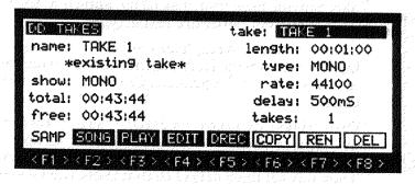
Here you may select takes and view their record parameters as well as select new takes for recording or deletion, etc.. To return to the main sample editing functions, either press F1 again (SAMP) or simply press the EDIT SAMPLE key.
