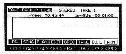
This page looks very much like the normal record page except that you have lost the threshold field. To perform a restore of either a single take or all takes, line the DAT up to the appropriate point and press ARM (F8) on the S1100. You will receive the following message:
