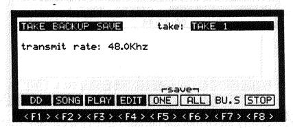
This simple page displays the transmit rate for the back up to DAT and can be set to 44.1 or 48Khz. When a take is backed up to disk, all data related to it is also backed up, of course. This includes start and end edit points, MIDI parameters, fade in/out, etc..
