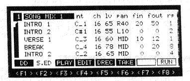
Normally, the takes will be recorded onto disk in sections, one by one, edited and then compiled into a song within the S.ED page. Here we see a series of such takes running back to back to form a typical extended remix. You can see that some
