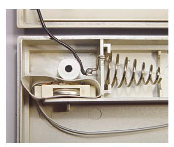
The battery and holder, within a tube of white plastic (which happens to be heatshrink, but has not been shrunk), ready for the machine to be re-assembled.
