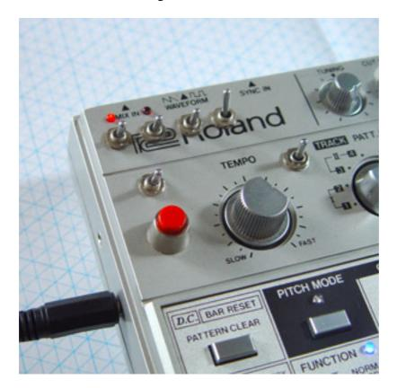
**32 Bank Memory system**: five toggleswitches and one pushbutton switch (the right toggleswitch is for a different modification – Audio In to Filter), for the TB-303 Devil Fish, with the **additional modifications for Dynamic Bank/Channel Switching**: Two 3.5mm sockets for Audio/CV inputs and two red LEDs to indicate the sockets' detector circuits being activated and so inverting the address bits generated by the two left-most toggleswitches.
