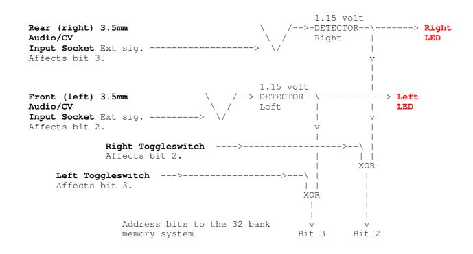
If nothing is plugged into the two Audio/CV Input sockets, then the detector circuits will be Off, the Red LEDs will be Off and the address bit inversion circuits (the XOR gates) will not invert the input they receive from the toggleswitches. So if the toggleswitch is down, the bit which forms part of the memory bank address will be 0, as it is for the other toggleswitches for bits 4, 1 and 0 (assuming the pushbutton is not pressed, since this inverts bit 4).
