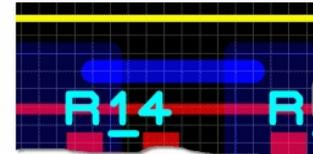
**⚠ Note that the BRIDGE track style is - of necessity - outside of the netlist and therefore ARES will not warn you if you make a mistake. Use with caution.**
