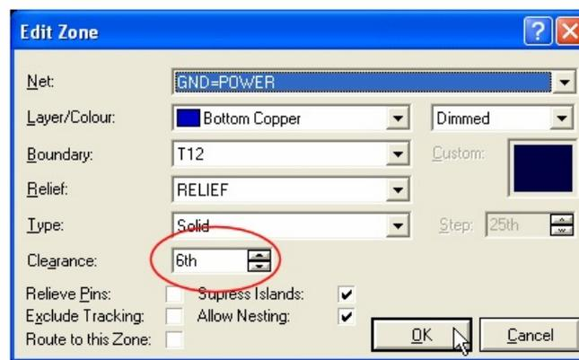
*Setting the clearance of a Power Plane*
