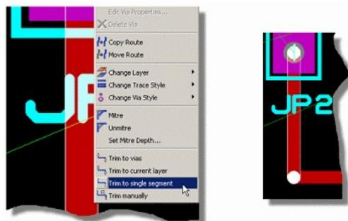
*Trimming the trace to a single segment*
