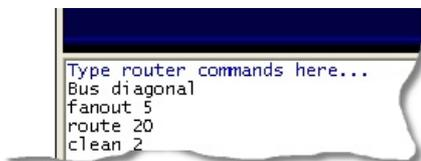
4. Subsequent routing phases consist of the [route command](#) (two parameters - number of passes and start pass) followed by the [clean command](#) to tidy up.
