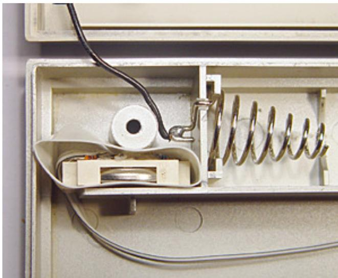
The battery and holder, within a tube of white plastic (which happens to be heatshrink, but has not been shrunk), ready for the machine to be re-assembled.
